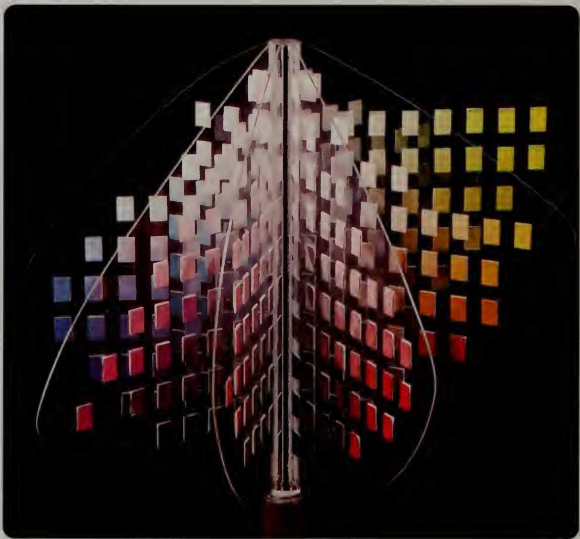
FIGURE 1. A photograph of a color solid constructed of Munsell samples affixed on ten constant-hue charts or vanes. Note that the hue changes as the solid is rotated about its vertical axis. This color solid was constructed at the National Bureau of Standards under the author's supervision.
